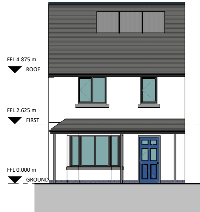
END TERRACE FRONT ELEVATION 1 : 100
